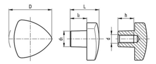
$\begin{array}{lll} D & = 40 \\ d & = M6 \\ d1 & = 14 \\ h & = 12 \\ L & = 26 \\ l2 & = 14 \\ Weight (g) = 94 \end{array}$
